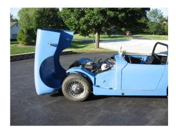
I also used Spitfire style latches for the front bonnet which work nicely with the Sebring front cutouts with minor modification to the latch bracket. The car has a 1275 with street cam and a 45 mm DCOE Weber with Pacesetter exhaust manifold and Monza exhaust. So gets along nicely, all be it a little fresh in the face with cool Fall weather in October. Unfortunately, with Extended Antique rego plates, we can only drive from April through October, so "Bluey" is currently hibernating for Winter!
